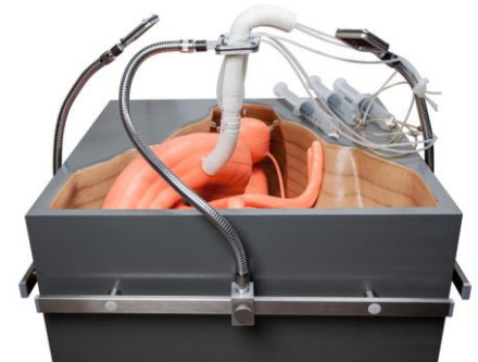
Figure 24: The new 2:1 scaled phantom model with the STIFF-FLOP arm entering through a trocar port
