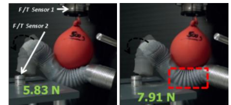
Figure 13: Examples of the 2-module manipulator interacting with water filled balloons and exploiting combined stiffening, dexterity, and force capabilities to perform surgical-like tasks.
