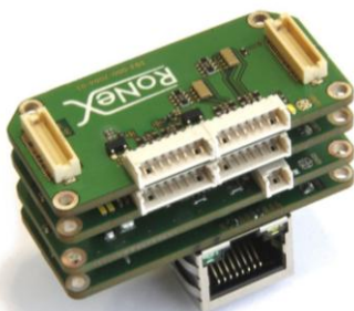
Figure 28: RoNeX Starter Kit, including one Bridge Module, one GIO Module and one Power Injector
